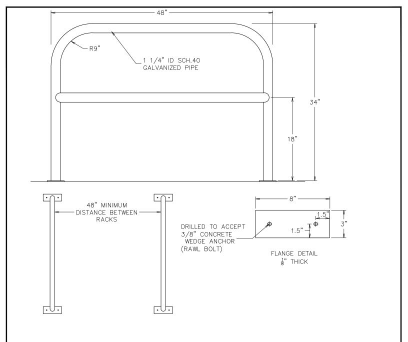
WELDING SHALL BE 100% AND WELDED WITH  $\frac{1}{4}$ " FILLET WELDS. FLANGE PLATE SHALL BE CENTERED AT 90 DEGREES TO THE RACK. ALL WELDS, FLANGE PLATES AND AREAS WITHIN 2" OF THE WELD SHALL BE TREATED WITH COLD GALVANIZING.
